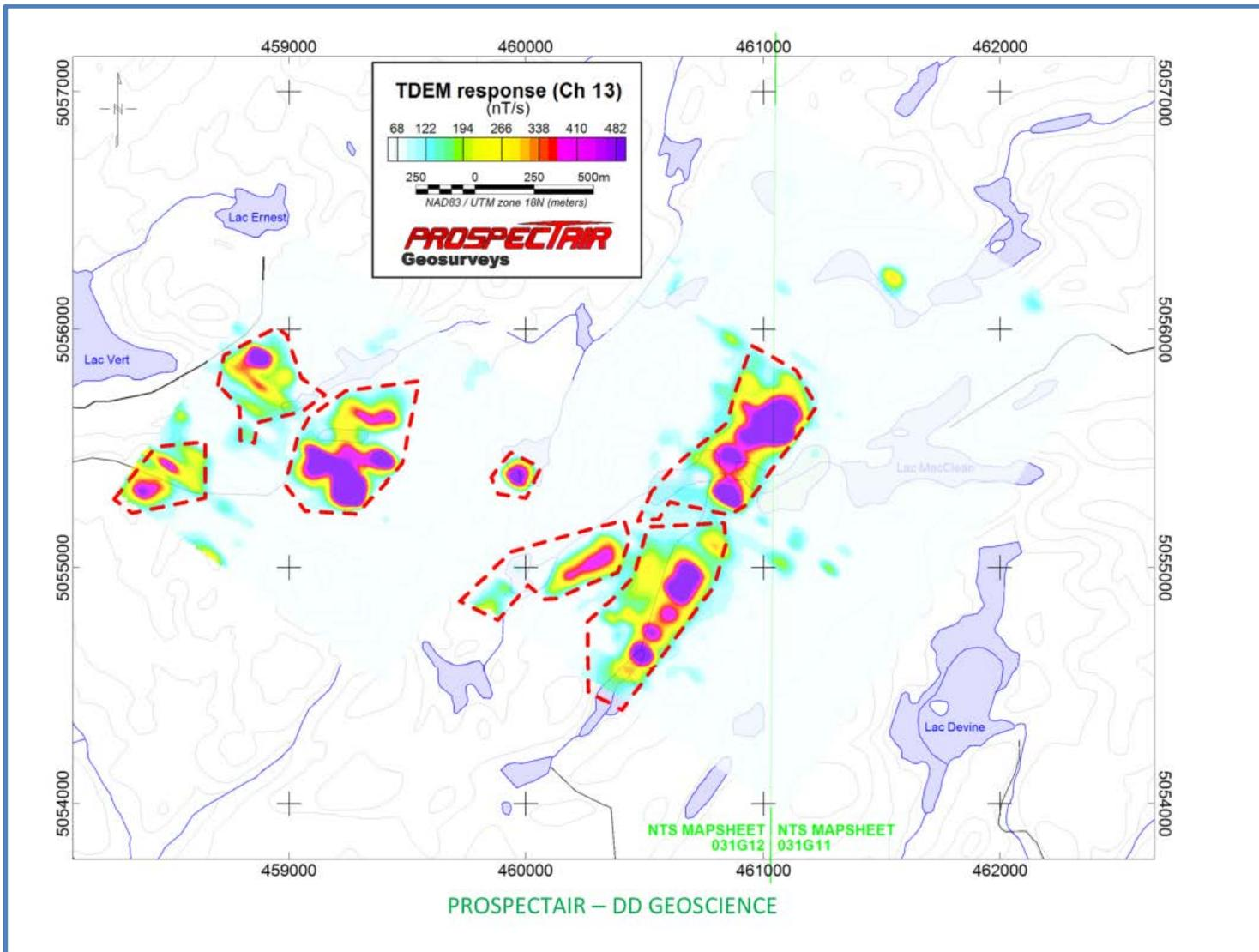
Figure 6. Heliborne EM and DTEM survey of 2013 (after Dubé 2013)
