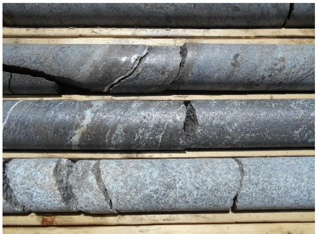
**Figure 13c)** Mineralized contact marble / paragneiss (BH16-04).
