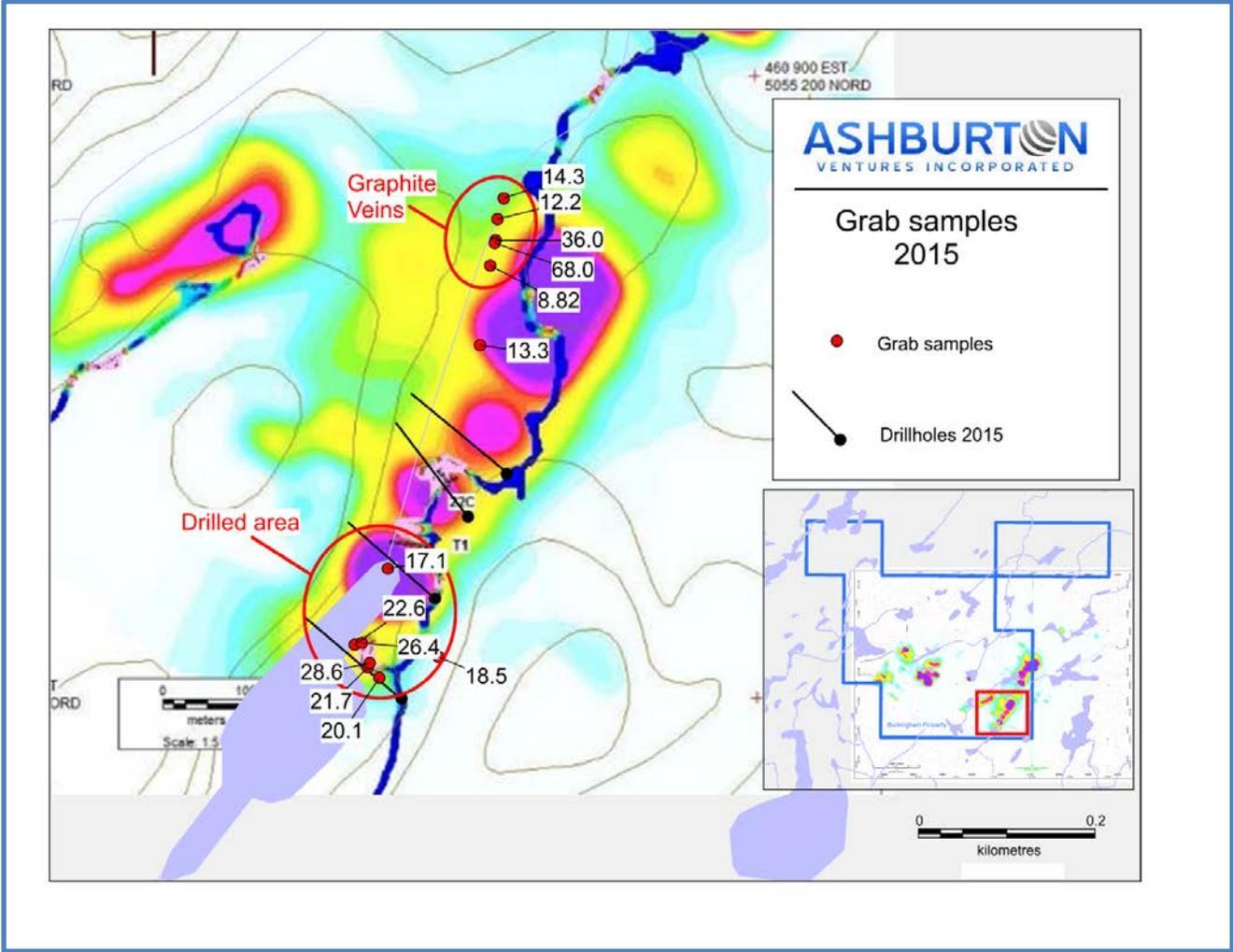
Figure 14. Locations of grab samples (2015) with respective percentage of graphite content
