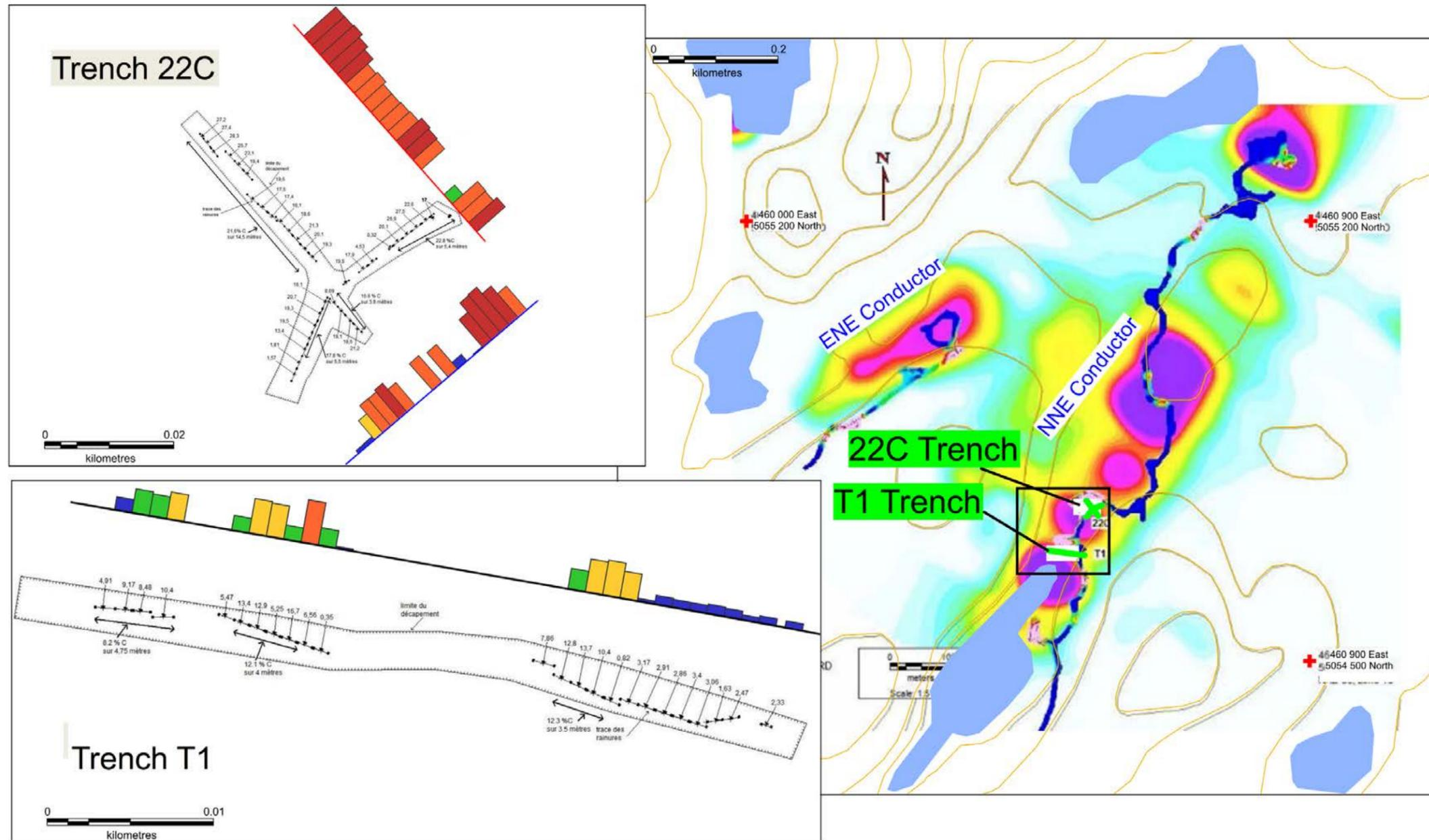
Figure 7. PhiSpy limited survey of 2014 with location of the sampled trenches (after Ouellet 2015).
