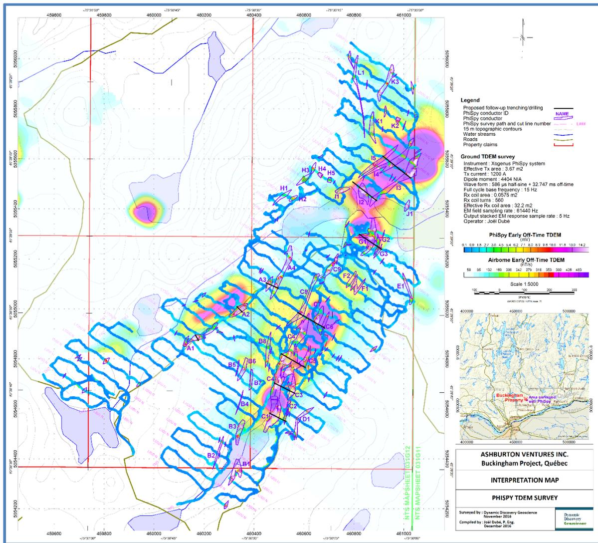
Figure 15. Ground PhiSpy survey and conductive zones, taken from Dubé (2016)
