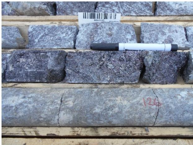
**Figure 13b)** Mineralized garnet-gneiss (BH16-01)
